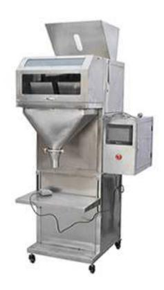
This machine is for packaging different kinds of granules such as seeds, fertilizer, salt, detergent powder, rice, sugar, etc.
