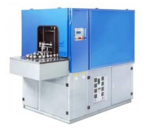
PET Plastic raw materials to make bottle embryo, and then blowing. The commonly used is the environmental protection plastic PET material. Using the machine to blow out of the wind, blowing PET plastic body attached to a certain shape of cavity, thus made products.
