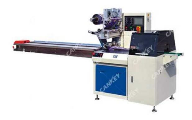
The horizontal popsicle wrapping machine is specially designed for the packaging of some bulk, soft, long strip materials without distinguishing between the positive and negative sides. The longitudinal sealing device is on the upper part of the package, which can alleviate the influence of heat sealing on the package.
