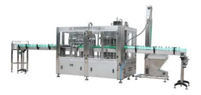
This rinser-filler-capper monobloc machine is mainly applied to pack juice, milk and other noncarbonated drink into glass bottle or PET bottle, its filing method is by negative pressure which produced by a vortex pump, and capper is suitable for twist off iron cap. This machine has advantages of higher automation and reliability in operation.
