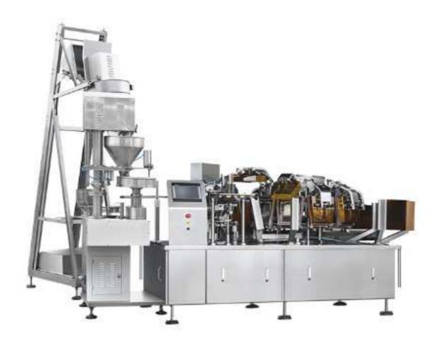
This is an automatic vacuum packaging machine, which provides full automatic production of bagmetering-filling-vacuum-sealing, avoids direct contact between employees and materials, saves labor, optimizes production processes, and eliminates pollution. Improve production efficiency and reduce costs. It can be used for mustard, sauerkraut, radish, mushroom, seaweed, etc.
