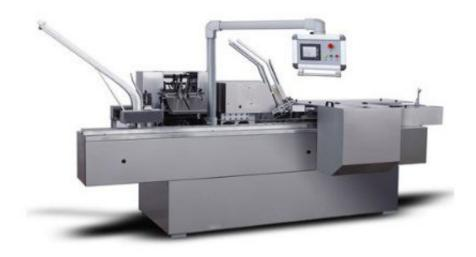
This is one of the perfect box filling machines with sound quality. The machine supply a box filling solution applied to Aluminum plate blister, bottle and soft tube in packaging of pharmaceutical, food, chemical and cosmetics. The latest and developed technologies adopted to this equipment ensure the speed and accurate work in stably.
