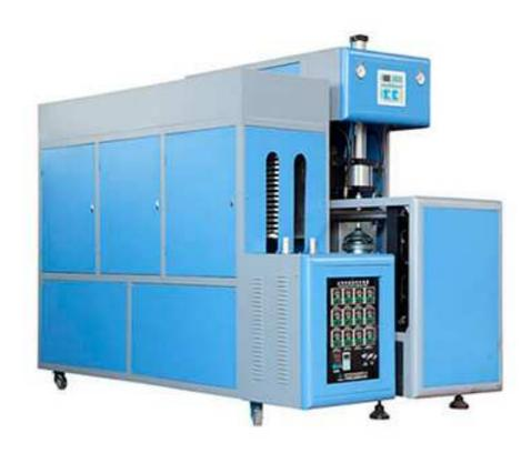
BM-9B semi-automatic bottle blow molding machine is suitable for producing PET plastic containers and bottles from 5L-10L. It is widely used to produce the carbonated bottle, mineral water, pesticide bottle oil bottle cosmetics, wide-mouth bottle etc.
