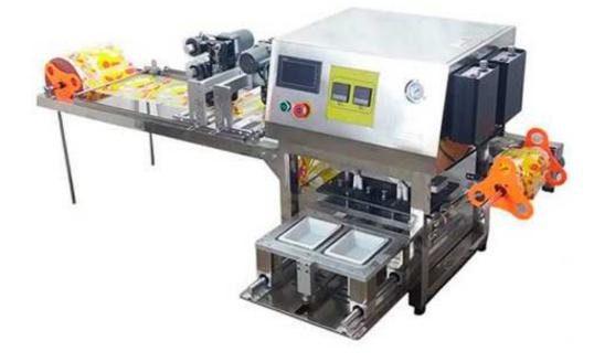
Automatic food tray top sealing film machine with date coder with date printer belong to automatic plastic tray box packing machine, the whole machine is made of stainless steel 201. Simple and reasonable structure, sealing of high efficiency and easy operation; Suitable for various sizes of plastic boxes, plastic trays and special-shaped plastic containers heat sealing, it's widely used in pharmaceutical, cosmetic and food industries.
