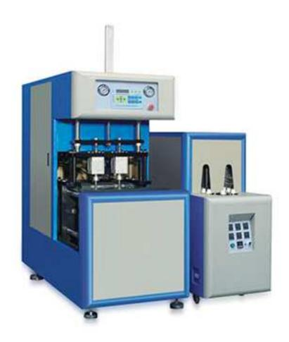
WBS-1-10 plastic Bottle Making Machine (semi-automatic Bottle Blowing Machine) blows bottle from 5L-10L. 5L 2cavity, 10L 1cavity. It is suitable to produce different shapes of water bottle and oil bottle. With low inverestment and easy operation, it is popular by customers.
