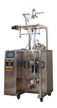
This machine can automatically measure; make bags, fill, seal, cut, and make easy tearing notches and can setting the fix number of cutting. Suitable for all kinds of liquid like tomato paste, wine, shampoo, jam, sauce, honey, oil, olive oil, hair gel and so on.
