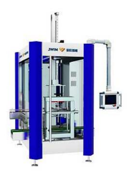
It is used for the carton packing and work with the logistic code system. This carton packing machine is widely used in the food, daily products, agrochemical and other industries.
