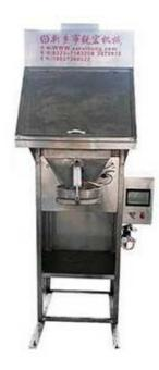
High-dose powder packaging machine is manually assisted in the bag, automatic weighing, bagging, filling, vibrating, pushing the bag, passing through the conveyor belt for automatic sewing or sealing. By changing the feeding mode, it is suitable for the quantitative packaging of ultra-fine powder to large-particle materials, such as rice, beans, milk powder, feed, metal powder, plastic granules and various chemical raw materials.
