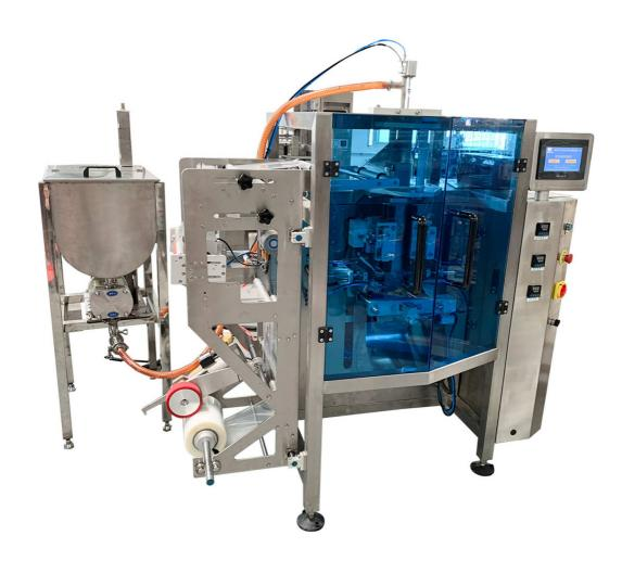
Automatic four-side sealing chili sauce packing machine includes servo rotor pump and reciprocating technology packing machine; Because the chili sauce has seeds and sesame which cannot be filled well by common liquid pump and reciprocating machine can work more stable.
