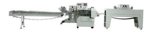
L-type High Speed Shrink Wrapping Machine is a fully automatic unattended wrapping machine, including automatic film feeding device and manual adjustment of punch guiding system and manual adjustment of feeding conveyor platform, matching with the packaging line. This machine can realize automatic feeding, bag forming, sealing, cutting and shrinking. It is suitable for products of different widths and heights, and also has the function of sealing, specially designed for packaging small products.
