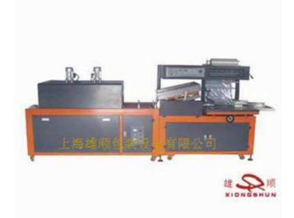
The machine adopt anti-viscosity, high temperature resisting, thermostatic super fine aluminumalloy sealing cutter. Adjusting precision of temperature and making bags length is super; the running is steady and dependable. It is suitable for film contraction packing in pharmaceutical, food, and toothpaste, cosmetics, electron and toy industry
