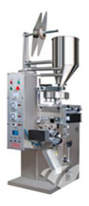
Model DXD10 Tea bag packing machine It is suitable for automatically packaging of steeping products such as fragmental tea, medicinal tea, coffee etc. The packaging bags with cotton thread. All the works of bagmaking. measuring, filling, sealing, cutting and counting can be done automatically.
