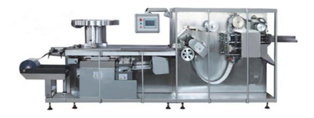
Roller-Plate type blister packing machine is a kind of blister aluminum (PTP) / plastic (PVC) compound sealing packaging equipment, It can pack the material like the drugs (tablets, capsules) food, medical equipment, health products, electronic components and so on, as using positive pressure forming, rolling sealing, it has a blister crisp, smooth forum features.
