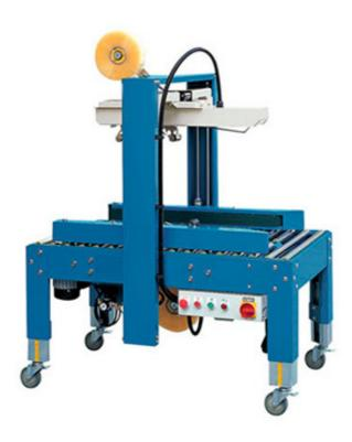
The CHS-6601A carton sealer is an automatically adjustable auto carton sealer which is easy to use and enables every operator to start operation and adjust different cases. We have designed and manufactured according to CE Machinery directives.
