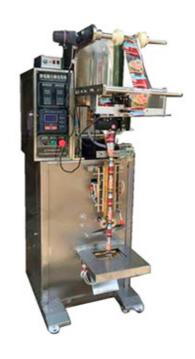
This ice Popsicle liquid filling machine uses microcomputer control system, the stepper motor controls the length of the bag, intelligent temperature controller (to ensure that the temperature error control within 1 °C). You can choose three-sided seal, four-side seal and back seal, to meet you requirements.
