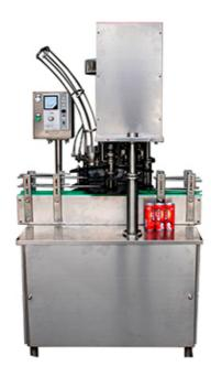
The seamer is mainly used to seal pop-top can of tinplate and aluminum alloy and PET can. It has four sealing positions with the seal component. Can revolve and circles around the main spindle when seamer is sealing.
