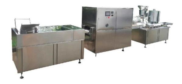
This production line is suitable for filling and capping Oral liquid, nutrient, energy drink, test agent, tube, medicine, liquid etc.
