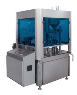
YSXZB Series automatic rotary preformed cup filling and sealing machine is applicable to pack the products like yogurt, milk, mineral water, beverage, ice cream, seasoning and so on. The process is from cup separating, sup falling, quantities filling, suck cap film, sealing, and product conveying. The choice of the machine model and number of filling heads depends on the factors like required output, size and type of packaging and requirements for additional equipment.
