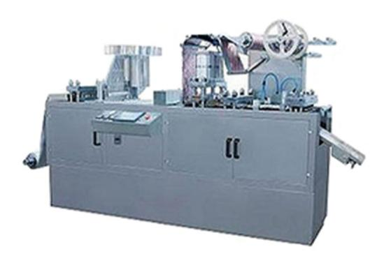
The machine is the latest generation product in our company adopting micro-computer PLC, frequency converter, and man-machine interface. It can check on-line and eliminate the waste plate by itself. In accordance with GMP rule requirement, it is an ideal blister packaging machine for aluminum-aluminum, aluminum-plastic, paper-plastic. And it has got high popularity. The products have been appraised as the provincial science and technology accomplishments.
