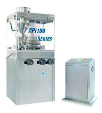
ZP1100 Series of Rotary Tablet Presses are the mid-range mass production capacity, which are widely used in the pharmaceutical, herbal, chemical and food industries to produce all types of round tablets and other irregular shapes tablets.
