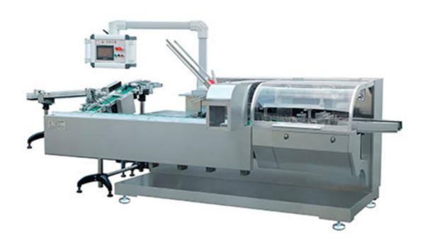
This machine is applicable for encasing ointment, injection and vial etc automatically. The working process is product conveying, leaflet conveying (1-4 fold), carton opening and conveying, box and leaflet encasing, meanwhile finish auto batch coding and carton sealing. (Hot melt glue device as option)
