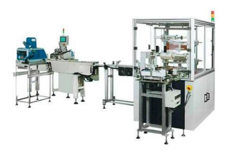
The fully auto model OSA-380 is good for hard square box. It adopts either shrinkable or non-shrinkable BOPP film to be folded on sides of box. It can have perfect packaging work without wasting trimming. Because of cheap price, it can save packaging cost & reduce labor cost. This machine is controlled by HMI, which is more human friendly without strict limitation by package sizes. The Auto Collator is an option to pack multiple products without needing box for cost saving.
