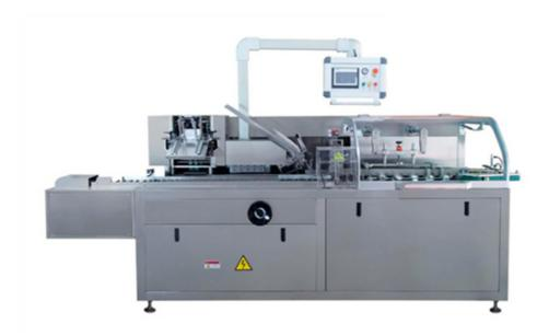
This machine is specially used for cartoning pharmaceutical bottles such as: ointment. Aluminum bottle and plastic bottle. The machine could fold the leaflet, open the carton and form ointment bottles automatically, these actions could bo finished by synchronization, the machine also could make the code printing on the catons. The machines is controlled by PLC.
