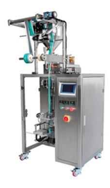
This machine is suitable for fully automatic round corner bag packaging of liquid materials in food, pharmaceutical, and other industries, such as coffee liquid, wolfberry puree, syrup, enzyme, honey, vinegar, and others. This liquid packaging machine employs specialized punching, sealing, and cutting techniques to enhance the sealing appearance of finished bags.
