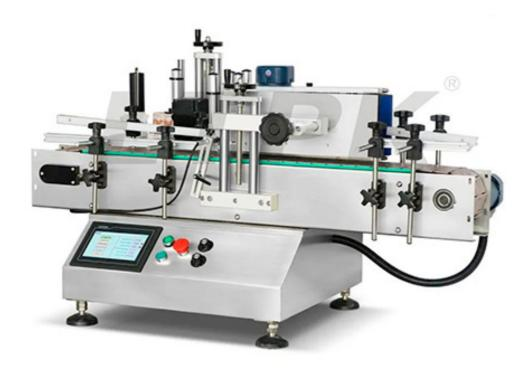
This is a tabletop wrap-around labeler designed to label cylindrical containers. It features a user-friendly interface and intuitive controls, making it easy to operate even for beginners. It is also designed for easy maintenance and cleaning, with a durable and long-lasting construction that ensures reliable performance for years to come. With the application belt, it can apply 3000 bottles per hour.
