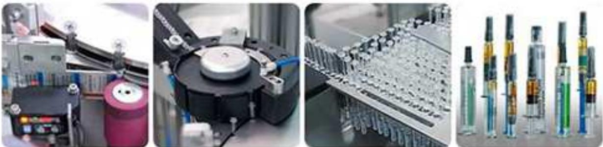
A11 is a specially designed machine for assembling the plunger-rod into and labeling on pre-filled syringes.
