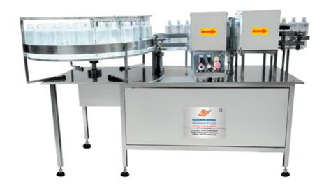
The Automatic Air jet Vacuum Cleaning System consists of a main structure, product loading conveyor, safety cover (OPTIONAL), product in-feed screw/star plate, inverter screw, pneumatic component, washing nozzles, electrical panel, AC drive & motor.
