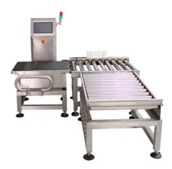
Large-capacity weight testing machine is automatic production equipment.
