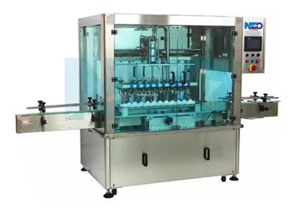
Automatic bottle filling machine having 12 head automatic liquid filling machine, filling machine capacity can be customized to suit production speed. This bottling filling machine can be used for bottling juices, oils filling line, honey, food products, pharmacy syrups, filling line, foamy liquids filling line, toilet cleaner filler, chemicals and any free flowing low to medium viscous liquids.
