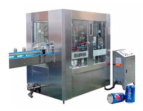
This machine is core machine in beer/carbonated drinks production line. It is for fill and seam of beer and other carbonated soft drinks (aluminum can/pet can), like cola, soda, energy drinks and so on.
