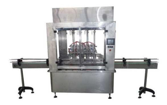
The machine is an automatic liquid filling device which is composed of PLC, human-computer interface, and optoelectronic sensor and air-powered. The machine adopts time control theory, switch time of the solenoid valve and metering pump to control the filling dose precisely. The machine is unique in simple operating, stable performance, accuracy measuring, no dripping or leaking and convenient in changing model.
