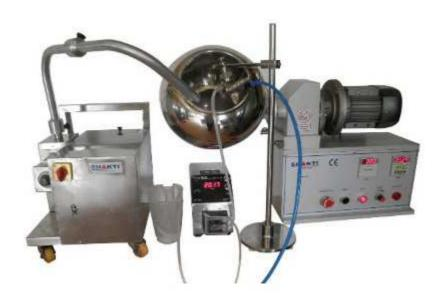
Coating with Peristaltic Pump, Spraying & Drying System: The Coating pan is used to produce uniform coating on tablets with the help of Baffles inside of pan. This can be mounting on the universal Gearing and as a result different tilting angle can be set up to 45 Degree. It is also permits speed control at any desired RPM. The pan capacity is 9.5 Liters Approx & Suitable to Attached in our Both Main Drive.
