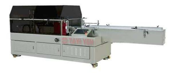
Package length is not limited. Packing rate varies with package length. maximum production is of up to 100PPM. (Small package)
