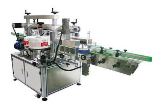
HL-T-502 Applicable to single side and double side labeling of flat bottles, round bottles and square bottles, such as shampoo flat bottles, flat bottles of lubricating oil, round bottles of hand sanitizer, etc. Double side labeling can improve production efficiency, widely used in cosmetic, cosmetics, petrochemical, pharmaceutical and other industries.
