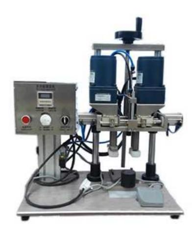
The desktop capping machine is suitable for the cap screwing of different shapes of bottles in the industries of foodstuff, pharmaceuticals, daily chemical, pesticide and cosmetics etc. Its four adjustable speed motors are used respectively for cap supplying, bottle clamping, delivering and cap screwing. It is characterized by high level of automation, outstanding stability, easy adjustment, no need of spare parts for replacing bottle types or caps, which can be done only by adjusting.
