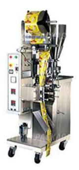
The MK-101 is an small automatic vertical form fill seal packaging (VFFS) machine designed to package granular and free flowing powdered products. This machine uses volumetric cup dosing system and is integrated with continuous type sealing system to produce center sealed, 3 side sealed and 4 side sealed pouches / bags.
