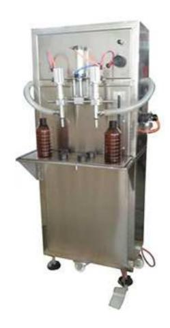
The machine adopts piston type quantitative filling principle, pure pneumatic operation, use the big bucket cylinder filling ingredients into the bottle, filling volume is adjustable and equipped with a mechanical anti-drip device, there are foot start and automatic continuous irrigation loading modes.
