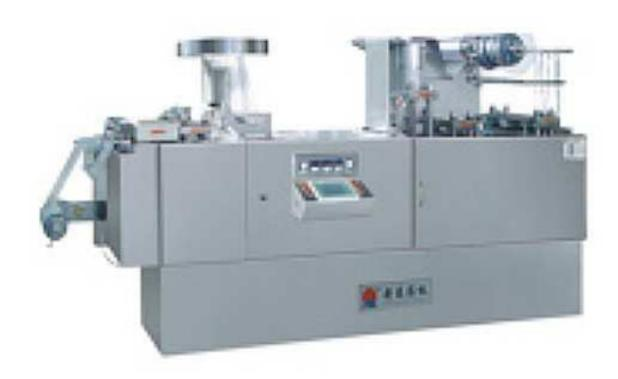
This product is a newly packaging machine designed for medicine in our company. Its function has reached domestic leading level; it is suitable for capsule, tablet, honey pill, candy, one injector and irregular-shaped AL/PL, Paper/Plastic and Al-Al sealing packing in pharmacy, food, electronics, medical equipment industry etc.
