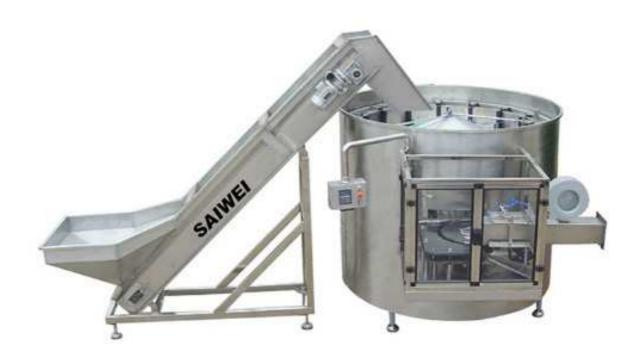
LP series rotary unscrambler is special designed as complete set for rinser/filler/capper monobloc and with the latest international technology. The bottles are transferee through neck guided air conveyor to the monobloc after unscrambling from the unscrambler with fast, high efficiency and sanitation, It is satisfied for high speed filling request, and also raise production efficiency of the whole line. The air conveyor can also be used for aseptic filling line after take some modification.
