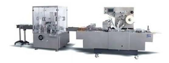
This machine is suitable for bottle (round, square bottle), into carton automatically. On line product feeding and detecting, carton opening and forming, products and leaflet push into carton, printing batch number, sealing carton with tuck-in or hot melt glue device. Automatically reject lacking of leaflet or product and finished product out.
