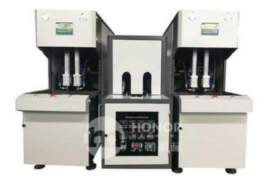
Bottle blowing machine is a kind of equipment which can make plastic granules into hollow containers by blow molding process. It is mainly used in beverage and food industry.
