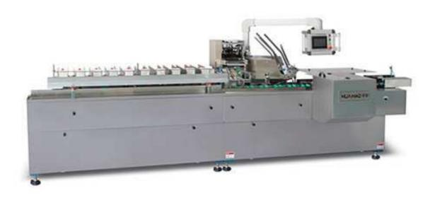
The product is suitable for cartoning and packaging of pain plaster, acupoint sticking products, facial mask, paste products, and similar goods, thus, folding of operating manual (1-4 folding), carton molding, goods loading, batch number printing, paper tongue sealing of both ends can be automatically finished. The machine can be used alone, and it also can be connected with other equipment for forming production line (Hot melt glue machine can be equipped).
