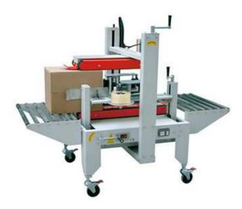
AS-423 side sealing case sealer is a special customized machine. It seals the mouths on the side of the carton and seals them at the same time. It is used for relatively flat carton sealing such as beverages, instant noodles and milk.
