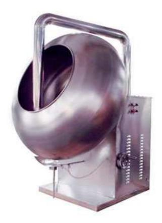
BY- 1250 Pan coating equipment, pan coating machine, chocolate panning equipment Introduction. This chocolate panning equipment is used for candy, chocolate or other granule foodstuff products. It is widely used in pharmaceutical or foodstuff industry. It is also suitable for granular material...
