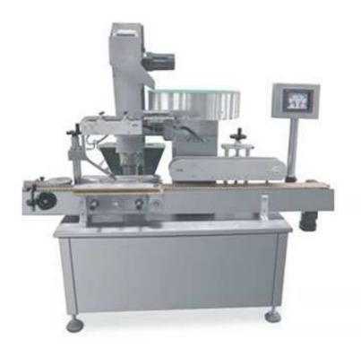
Equipped with three pairs of friction wheels, self-adjust tightness, helpful the caps surface. Wide applicability, it is simple and convenient if change bottles and caps, just, adjust some components. Equipped with human-computer interface and PLC control system, Ensure more stable operation and easier handling. Self-diagnose errors and stop working to make alarm at errors and missing bottles caps. The bottle with twisted cap, anti-cap and without aluminum foil will be removed.
