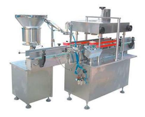
This plastic bottle screw capping machine has employed automatic cap feeding mode, electromagnetic oscillation for sorting caps, and constant torque for screwing caps. And its main components include conveying system, capping system and control system.
